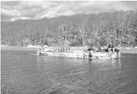
Below: Here are three photos of the shuttle scows that transport the material between the in-river dredge and the larger scow out on the mooring.
